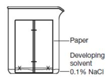
In this lab, we will separate food coloring into its component dyes by paper chromatography. Food dyes are spotted onto chromatography paper. The paper is hung into a beaker with a small amount of developing solvent, as shown to the left. As the solvent moves up the paper by capillary action, it carries food dye components with it. The most polar components move fastest, while less polar components move more slowly or not at all.
